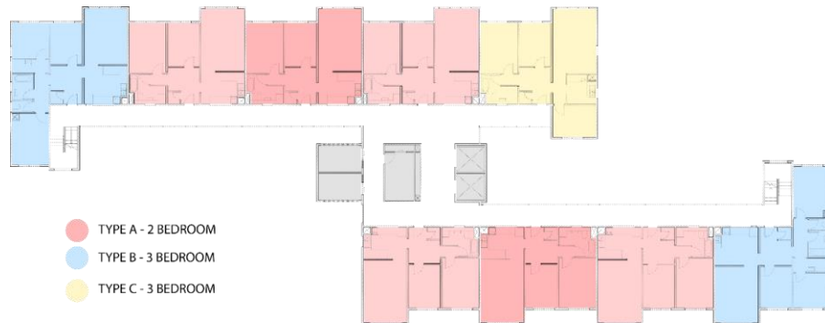
The existing layout of each floor is identical, with all flats having a window to each room and cross ventilation. In total there are 180 units per tower. Image by OFFICE.
