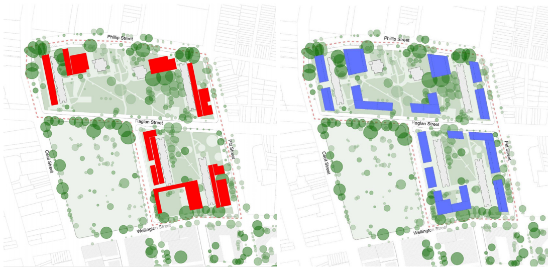
Figure 32: Existing carparks (red) make up a significant portion of the site. By locating new infill (blue) in these areas with carparking below existing trees and open space can be retained.
