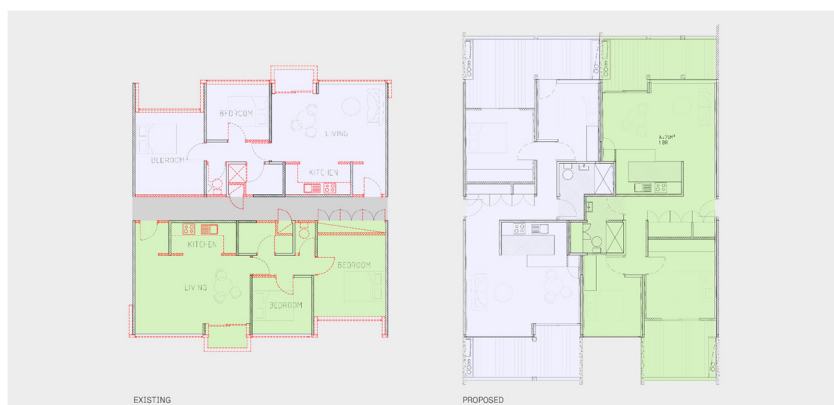
Figure 21: The central units are reorientated to eliminate the central corridor and provide the dwellings with dual outlooks and cross ventilation.
