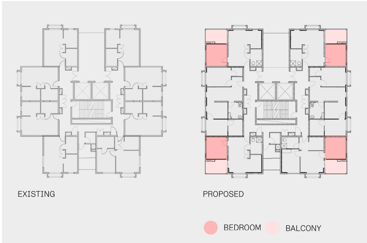
Figure 13: Typical plan of the tower highlighting the addition of a replicable bedroom and balcony module. This prefabricated addition turns the studio apartments into one-bedders.
